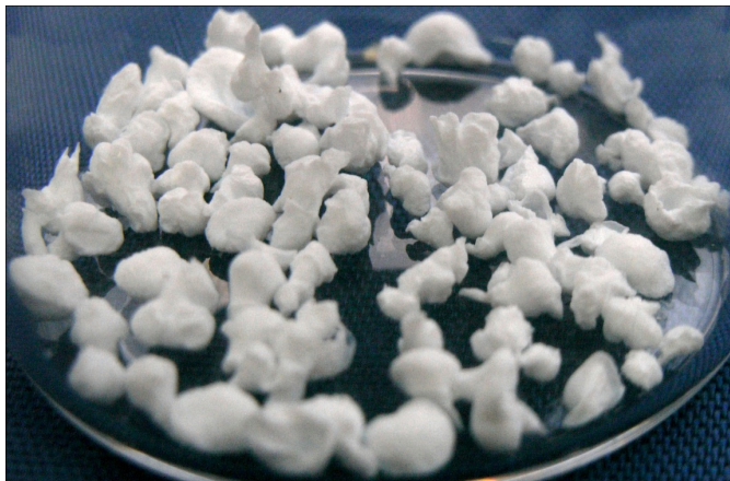
Figure 1.12 sPS nanoporous \delta form aerogel beads in the size range 100-1000 \mu\text{m} .
