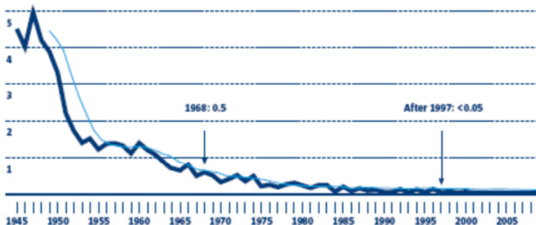
GLOBAL PASSENGER FATALITIES PER 100 MILLION PASSENGER MILES, SCHEDULED COMMERCIAL AIR TRANSPORT OPERATIONS, EXCLUDING ACTS OF UNLAWFUL INTERFERENCE
