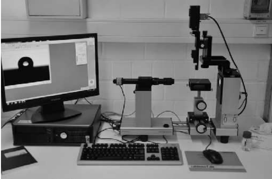
Figure 33: Contact angle system Dataphysics OCA20 present at the ENEA Research Centre in Portici.
