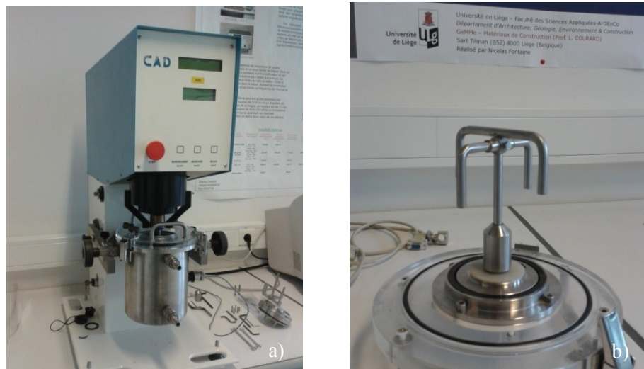
Figure II.11 a) RheoCAD 200 and b) anchor-like stirrer
