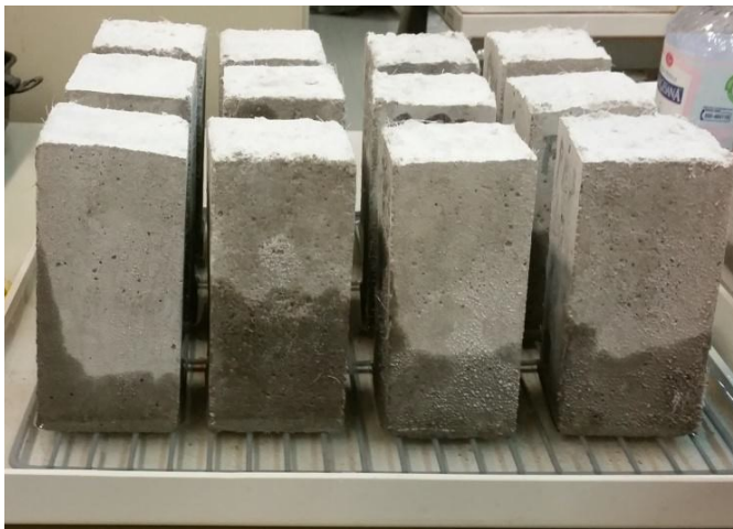
Figure IV.30 Example of water capillary raise in mortar specimens
