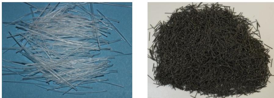
Figure II.8 a) PP fibers and b) Recycled+2FA foamed fibers
