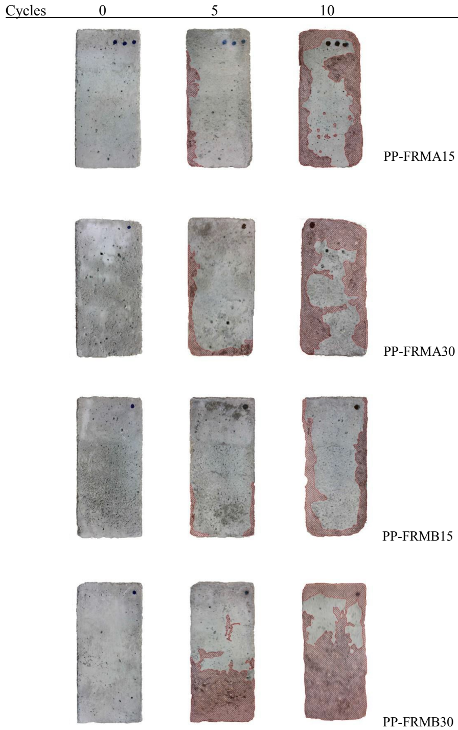
Figure IV.34 Comparison of the superficial degradation of PP fiber reinforced mortars at different cycles
