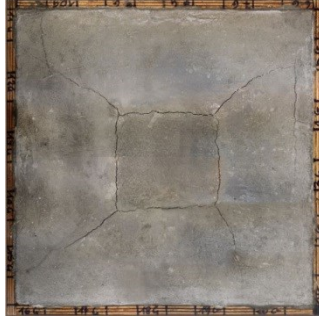
Figure IV.37 Reference panel at the end of the test (8 hours) (Coppola et al. 2016b)
