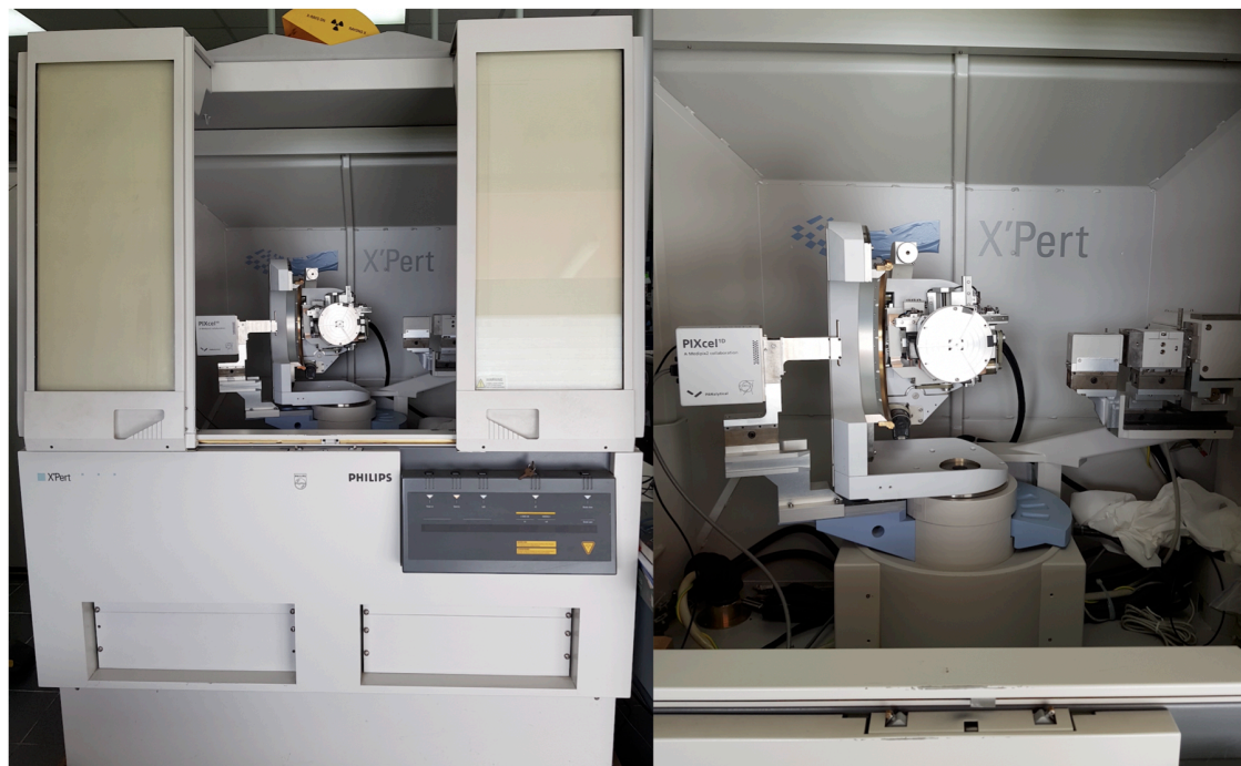
Fig. 2.3: The Philips X'Pert-MRD high-resolution analytic diffractometer at the M.U.S.A. laboratory CNR-Salerno. On the right, there is a zoomed image that shows the complex apparatus of this system.
