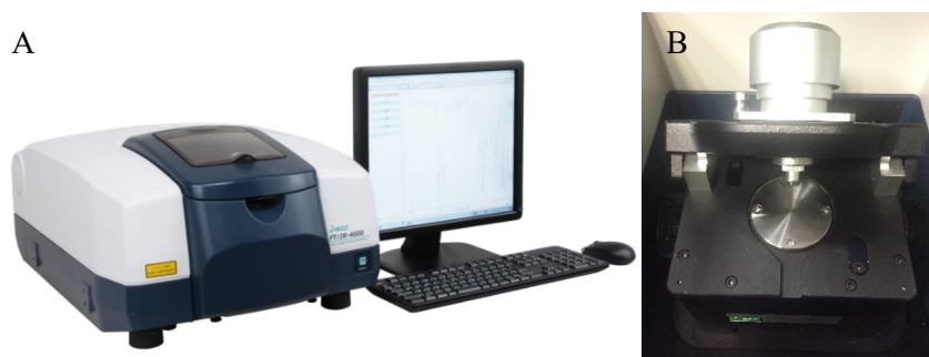
Figure III.5 FTIR spectrometer (FT/IR-4100, Jasco Corporation, Kyoto, Japan) (A) coupled to an attenuated total reflectance (ATR) device (B).
